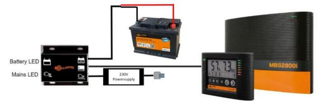
When connected to the system, both mains and battery LED will be illuminated green indicating both power sources are connected. In the event of mains failure, the mains LED will turn off and only the battery LED will remain on indicating the system is operating on battery.
